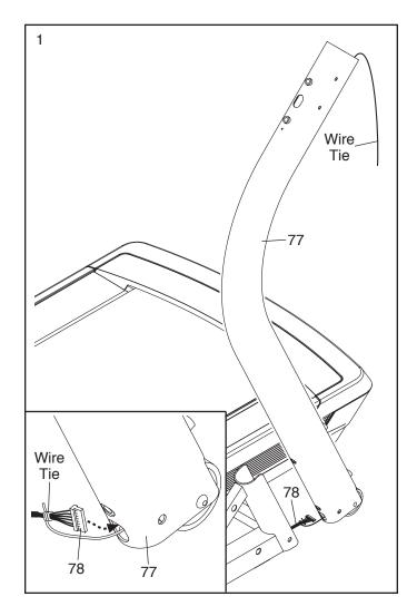
Attach the Upright (77) to the Base (80) with two 3/8" x 5 1/2" Screws (5), two 3/8" Star Washers (8), and a 3/8" x 2 3/4" Screw (17) with a 3/8" Star Washer (8) as shown. Start all three Screws, and then tighten them. Be careful not to pinch the Upright Wire (not shown) in the Upright.
